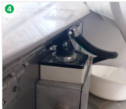
The metal container is equipped with a temperature probe in the lid of the base bath. In the event of a fire, this temperature probe disables the power supply causing the lid of the fire-box to close.
