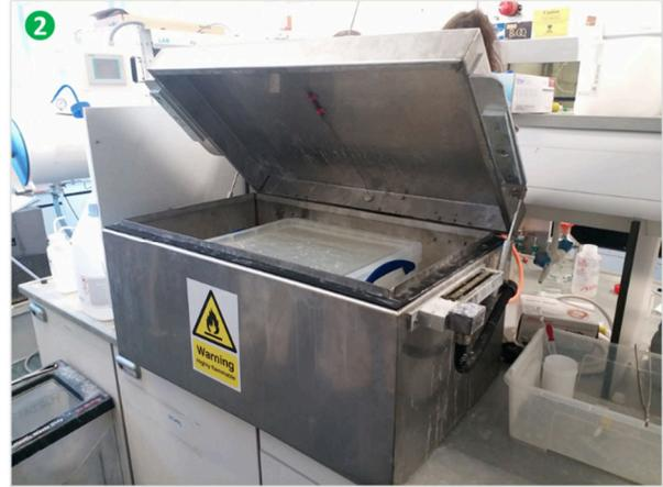
The default position of the box is closed (photo 1) and the lid should only be opened (photo 2) when adding or removing items from the base bath. As soon as you have finished working with the base bath, you must close the lid.
