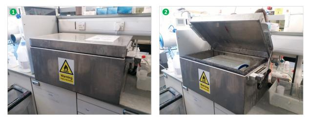
The default position of the box is closed (photo 1) and the lid should only be opened (photo 2) when adding or removing items from the base bath. As soon as you have finished working with the base bath, you must close the lid.
