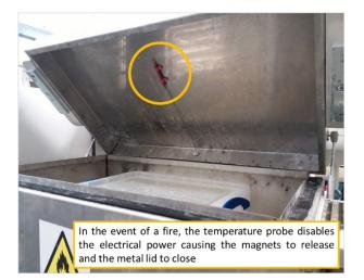
Any malfunction of the magnetic mechanism of the metal fire-extinguishing base bath should be immediately reported to the School Safety Coordinator.
